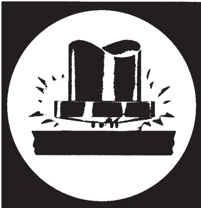
3. STUD FORCED INTO MOLTEN METAL.
