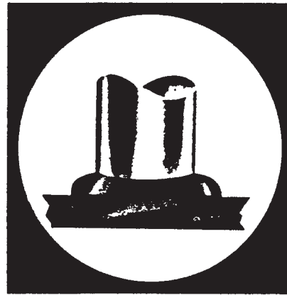
4. METAL SOLIDIFIES AND WELD IS COMPLETED IN MILLISECONDS
