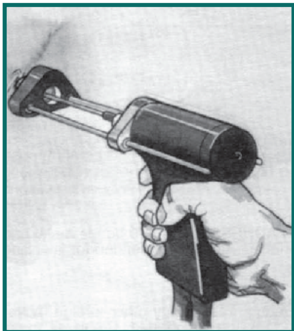
1. WELD PINS IN PLACE.
